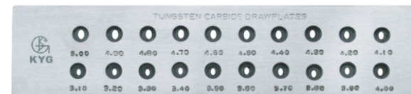
KYG1155 巨型(20孔)Egg—20 holes No.3.10-5.00 Size:208×46×7.5mm
