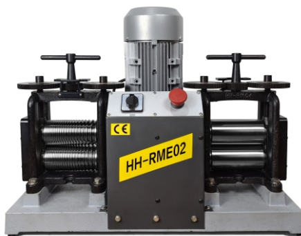
KYG0827 台式电动压片机(有拉线器) Electric Rolling Mill 电压(Voltage): 220V 功率(Power): 750W 滚轴直径(Roller Diameter): 68mm \times 160mm 长方槽(Cuboid): 1.5/2/2.5/3/4/5.5/7mm 半圆槽(Semicircular Groove): 5/6/7/8/10mm 压片宽(Width of Pressing Surface): 65mm 机身尺寸(Size): 400 \times 200 \times 490mm Weight: 50kg
