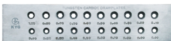
KYG1146 六角型(20孔)Hexagonal—20 holes No.5.10-7.00 Size:208×46×7.5mm
