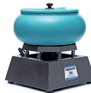
KYG0341 17寸震动抛光机 17 Inch Vibratory Tumbler 机身尺寸(Dimension):390x390x500mm 包装尺寸(Dimension):450x450x540mm 桶直径:430mm 电压Voltage: 110-220V 容量Capacity: 13L 重量weight: 19kg
