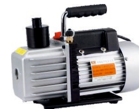
KYG0579 真空泵TW-1A Vacuum Pump 电压(Voltage): 220V/50Hz 功率(Power): 150W 电机转速(Motor speed): 1440rr/min 抽气速度(Pumping speed): 1L/S 真空度(Vacuum degree): 10Pa 加油量(Refueling quantity): 250ml 外形尺寸(Outline dimension): 270 × 120 × 235mm 重量(Weight): 5.7kg
