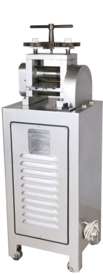
KYG0819 钻石牌电动压片机(1.5HP) Electric Rolling Mill 功率Power: 1.5HP/0.75KW/220V 滚轴直径(Roller Diameter): \phi 75mm \times L140mm 方槽(Square Groove): 0.8/1/1.2/1.5/2/3/4/5/6/7/8mm 压片宽度(Tablet Width): 75mm 轧辊转速(Roller Speed): 16r/min 轧辊材料(Roller Material): Cr12Mov HRC: 61-63 轧片厚度(Thickness of Rolled Sheet): 0.08-6mm 机身尺寸(Size): 350 \times 425 \times 1080mm Weight: 145kg
