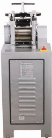
KYG0822 KYG电动压片机(1.5HP) KYG Electric Rolling Mill 功率Power: 1.5HP/1.1KW/220V 滚轴直径(Roller Diameter): \phi 68mm \times L140mm 方槽(Square Groove): 0.8/1/1.2/1.5/2/3/4/5/6/7/8mm 压片宽度(Tablet Width): 75mm 机身尺寸(Size): 350 \times 425 \times 1080mm Weight: 123kg
