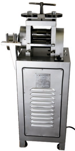
KYG0820 钻石牌电动压片机(2HP) Electric Rolling Mill 功率(Power): 2HP/1.1KW/220V/380V 滚轴直径(Roller Diameter): \phi 80mm \times L152mm 方槽(Square Groove): 0.8/1/1.2/1.5/2/3/4/5/6/7/8mm 压片宽度(Tablet Width): 82mm 轧辊转速(Roller Speed): 16r/min 轧辊材料(Roller Material): Cr12Mov HRC: 61-63 轧片厚度(Thickness of Rolled Sheet): 0.08-6mm 机身尺寸Size: 450 \times 400 \times 1300mm Weight: 175kg
