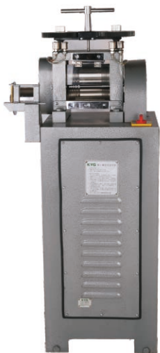
KYG0823 KYG电动压片机(2HP) KYG Electric Rolling Mill 功率(Power): 2HP/2.2KW/220V/380V 滚轴直径(Roller Diameter): \phi 83mm \times L160mm 方槽(Square Groove): 0.8/1/1.2/1.5/2/3/4/5/6/7/8/9mm 压片宽度(Tablet Width): 82mm 机身尺寸(Size): 400 \times 450 \times 1250mm Weight: 180kg
