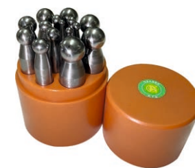
KYG1095 套装冲头(大15支) Dapping Punching With 15pcs Big Size:Φ4/5/6/7/8/9/10/11/12/13/14/15/ 16/17/18mm Weight:1149g
