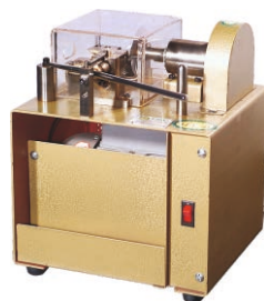
KYG0695 切割机(大)(TSK4023) TSK Tube Cutting Machine-Large Size:260 × 230 × 308mm Weight:16kg 可切割物件长度(Cutting In Length):30mm 可切割最大直径(Cutting In Diameter):12mm
