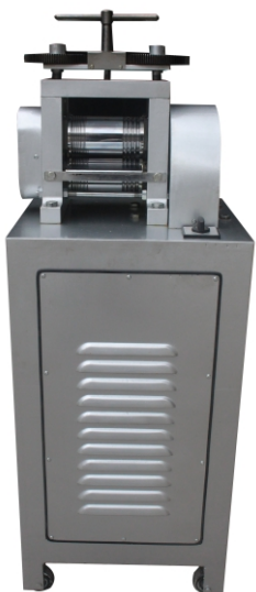
KYG0821 钻石牌电动压片机(3HP) Electric Rolling Mill 功率(Power): 3HP/1.5KW/380V 滚轴直径(Roller Diameter): \phi 86.5mm \times L165mm 方槽(Square Groove): 7-11mm(共12条) 压片宽度(Tablet Width): 82mm 轧辊转速(Roller Speed): 18r/min 轧辊材料(Roller Material): Cr12Mov HRC: 61-63 轧片厚度(Thickness of Rolled Sheet): 0.1-7mm 机身尺寸Size: 500 \times 430 \times 1350mm Weight: 200kg
