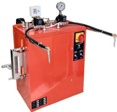
KYG0435 17L快速蒸汽清洗机(自动加水) 17L High Speed Steam Cleaner 17L/7KW/380V 机壳尺寸(Iron Sheet Size):300x450x560mm 外观尺寸(Dimension):490x530x730mm Weight: 61kg 设有直接抽水后成高压蒸汽冲洗，无须等待时间，工作效率高。 Equipped with facilities that can pump water directly and turn it into high pressure steam for washing.No need to wait and high efficiency
